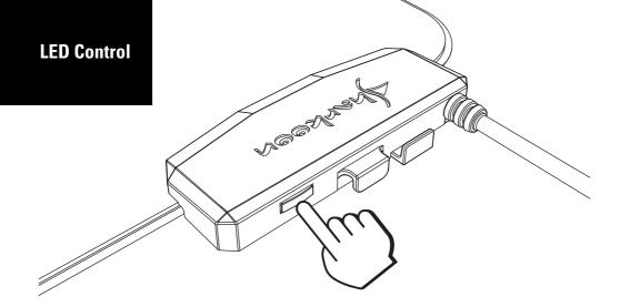
With the lighting off, press the button on the controller twice in quick succession to activate the illumination. Permanent is the preset mode, while green is set as the default color. Press the controller button once to change the color. The color sequence is as follows: green, red, blue, yellow, light blue, purple and then white. Press and hold the controller button to dim the illumination. Press the controller button twice in quick succession to switch to the next lighting mode.
